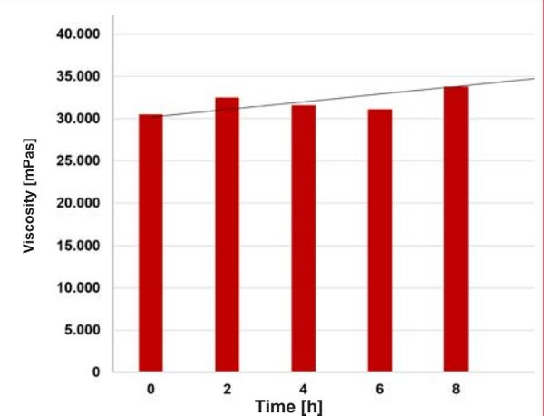
We recommend that once molten, the adhesive should be processed within 4 hours.
